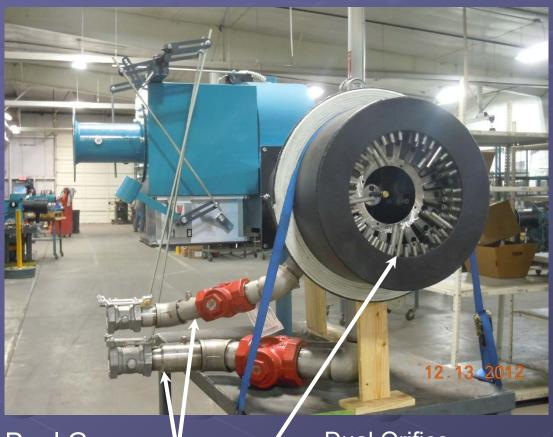
Dual Gas Piping Dual Orifice Comb Head
