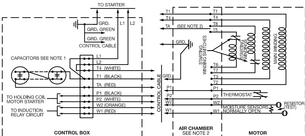
**NOTE 1:** CAPACITOR CONNECTIONS: CONNECT IN SERIES AS INDICATED BY SOLID LINE FOR HIGH VOLTAGE AND IN PARALLEL AS INDICATED BY BROKEN LINES FOR LOW VOLTAGE.
