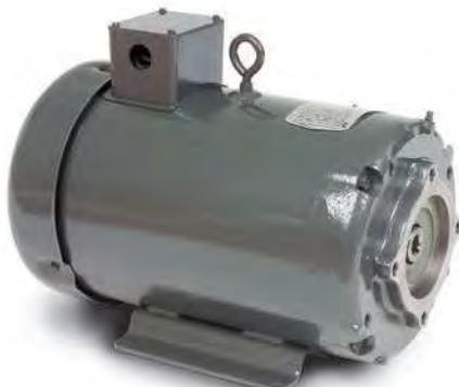
Baldor SEA Hydraulic Pump mount motors are designed to mount into hydraulic pumps for lifts, trash compactors and other machinery. They include a rigid base mount with SAE A or B pump mount face and shaft. The conduit box is F3 top-mounted for easy connections. These motors are designed for continuous duty but may also be used on intermittent duty applications. Their electrical design includes a robust Class F Insulation and 1.15 Service Factor.
