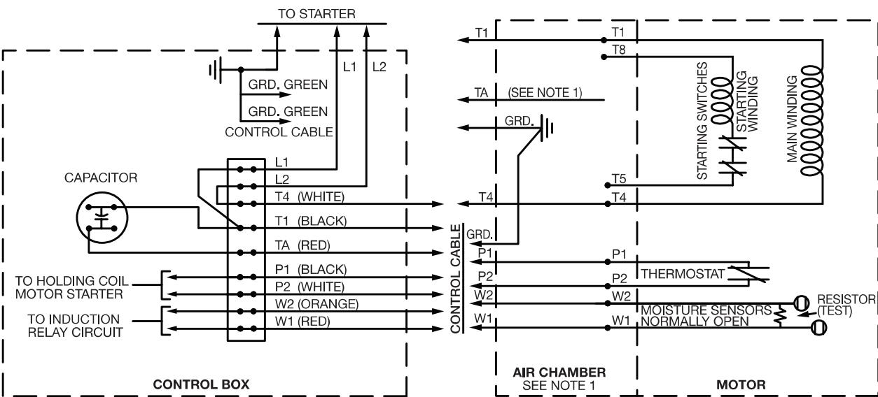
**NOTE 1:** IN MOTOR AIR CHAMBER CONNECT FOR DESIRED ROTATION PER WINDING DIAGRAM BELOW.
