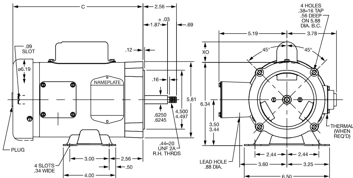
**Note:** XO = 1.56 on type 34L motors with a single capacitor. XO = 2.31 on type 34LC with dual capacitors.
