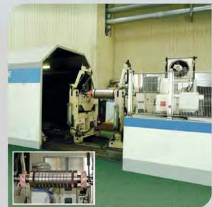
All rotors are balanced at operating speed using a high speed balance machine ensuring low vibration.
